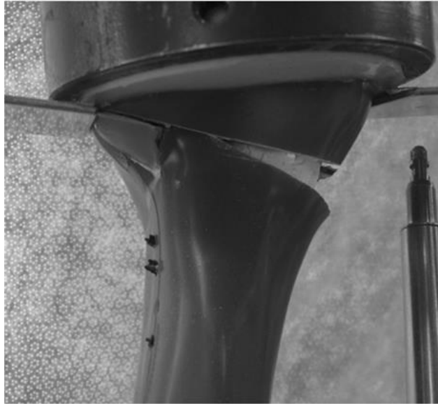
Figure 5.4: Example of lateral cortex fracture and osteotomy collapse
