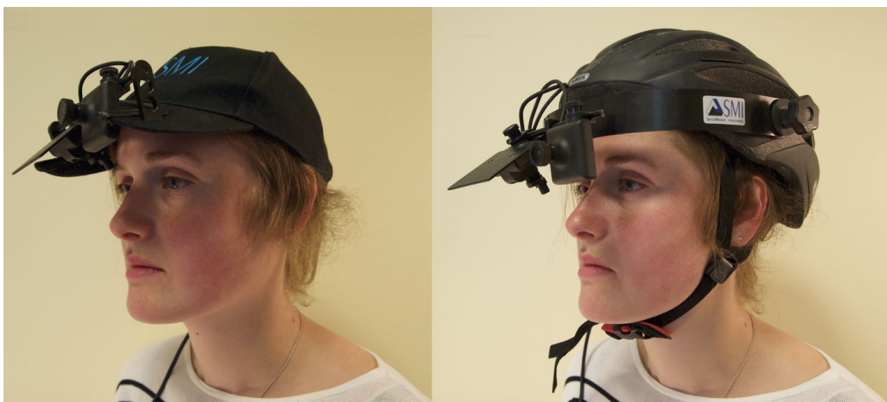
Fig. 1. Photos showing how the eye tracker was mounted in each of the two conditions: to a baseball cap (left) and a bicycle helmet (right).
